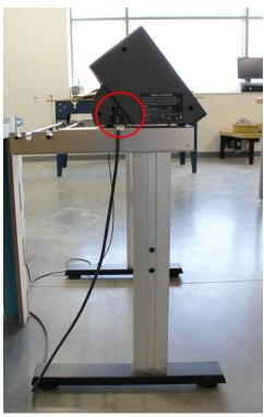
**Step 2:** Lower the media lever behind the operational keypad. This will release the pusher rollers for you to insert your media.
