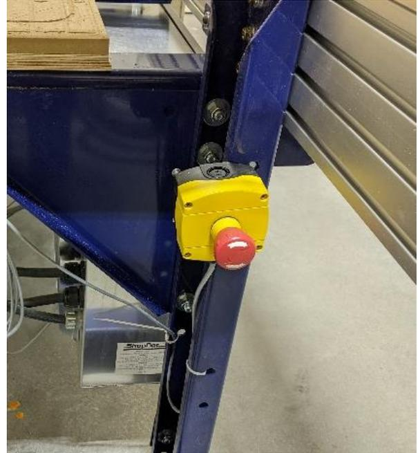
To activate the emergency stop press down on the red button. If you activate an emergency stop ask for assistance from NIS Staff immediately. Activating the emergency stop is a last resort. All job progress will be lost. Pause the job by using the space if possible.
