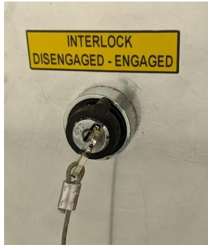
To arm the spindle, or allow the spindle motor to spin, insert the interlock override key into the keyhole in the control box of the Shopbot and turn the key  $\frac{1}{4}$  turn clockwise to “ENGAGED”. Note that this key can be overturned and underturned, both of which will not allow the spindle to turn. Do not over rotate key or damage will occur.
