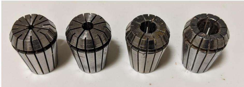
2. Remove the collet from the collet nut by pressing the collet out while simultaneously pulling the collet down. Consult with NIS Staff for stuck collets.
