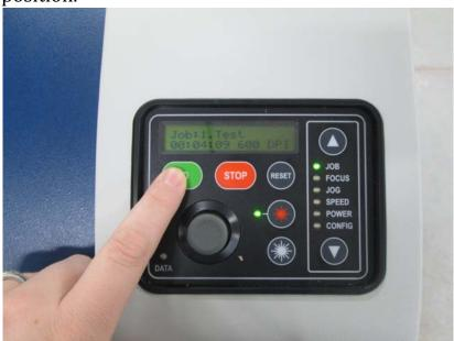
• The lid and front panel need to be closed to engage the laser. If you try printing with either of these doors open the laser will not fire and the print driver will go through ghost motions of your print.
