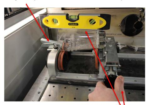
• Level your object by placing the micro level on the area you will raster and adjust the leveling wheel to raise or lower your object until it is evel.
