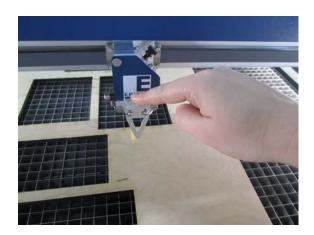
• When you reach the surface of your material with the manual focus tool **press down on the joystick once to set your new focus position**. Screen should read 0.00
