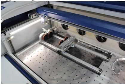
• Plug connectors in on the inside right side of the laser bed area, making sure that connector tabs are facing you.
