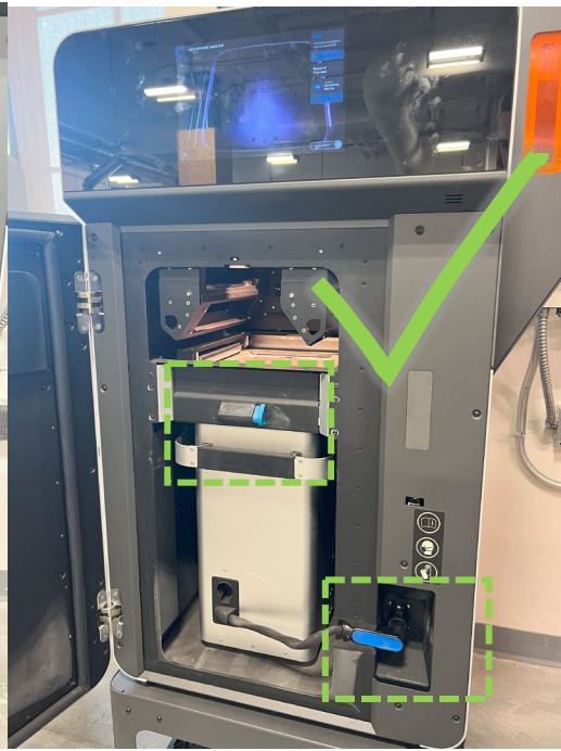
Latch is fully closed and plug is correctly seated
