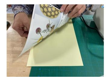
4) The yellow laminator sheets are slightly longer than the decal paper. Cut off the excess. Failure to cut this off risks a jam in the laminator.
