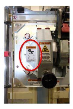
• Locate the 2 indexing pins on the front on the saw carriage housing.
