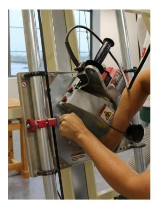
Make sure that both pins lock into the pin locators.
