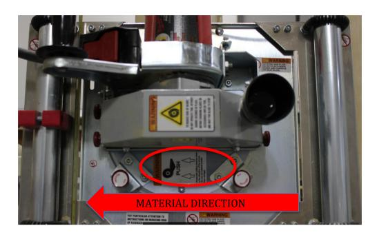
• Pull both pins outward (toward you) and swivel the saw body either clockwise or counter clockwise so that your cut direction corresponds with the arrows.
