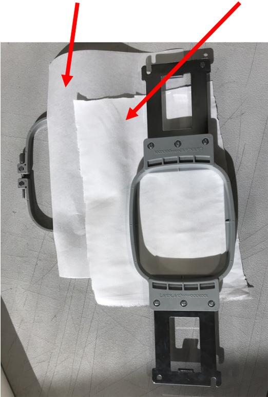
Press the larger hoop over the smaller one and pull the fabric and stabilizer taut like a drum . The bottom half of the hoop has a screw to tighten the hoop. If the fabric is too loose in the hoop, it can cause your project to fail or the needle to break.
