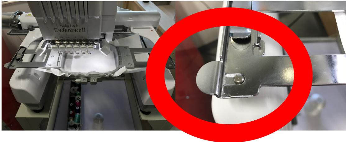
If you need to adjust the Baby Lock to accept a larger or smaller frame, loosen the two screws on the back left and slide the assembly to fit the frame. When you tighten those screws, hand tightening is sufficient.
